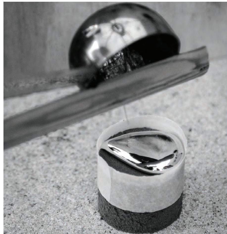
Figure 8. Pouring pewter in oasis. Photo credit: Anders Møller
