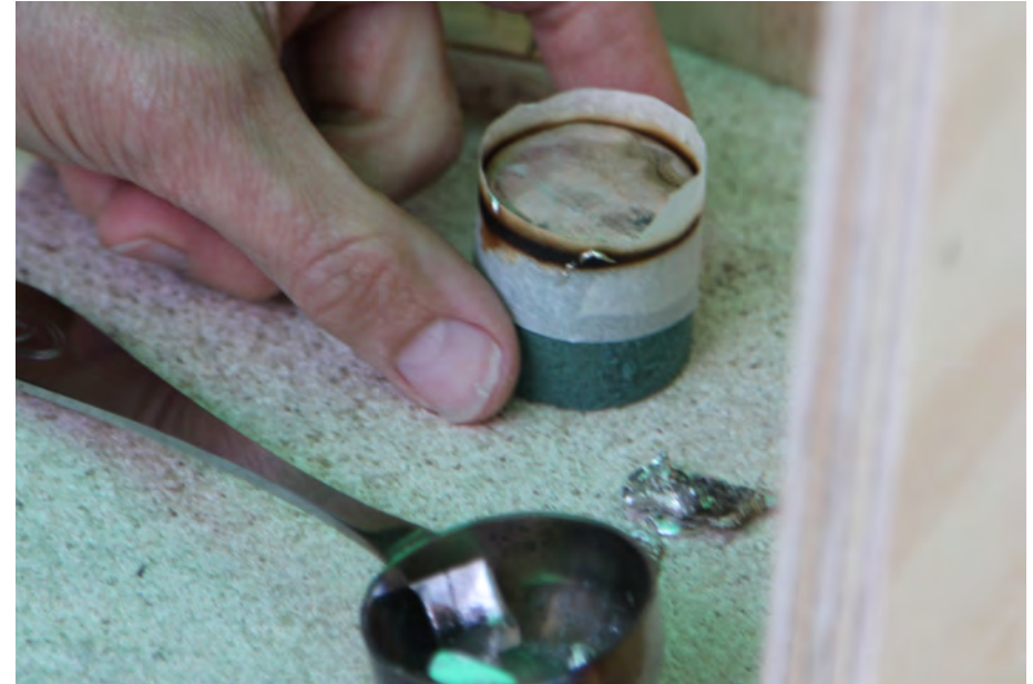
Figure 6. Casting pewter in oasis. Photo credit: Anders Møller
