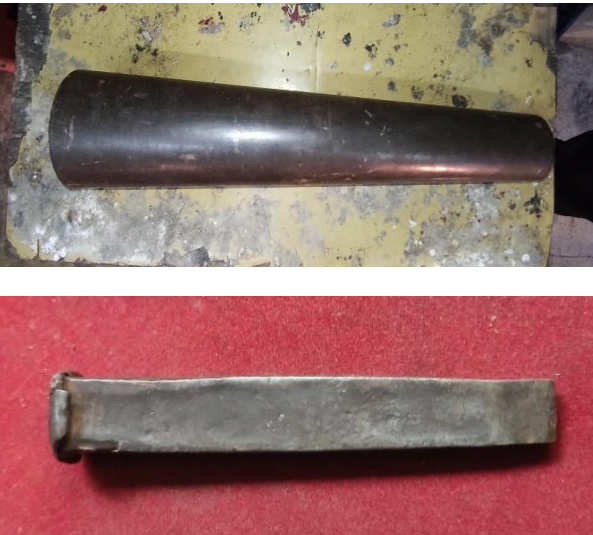
Fig. 26 (top) Kangan shail is used by jewellers to shape and adjust bangles into a uniform circular form during the bangle-making process. Location: workshop of Mr Ram Bharose Lal Verma and Mr Rajesh Kumar Verma, Bada Bazar, Nainital, Uttarakhand, 2024. Photo: Sah and Singh Bhakuni, 2024, under the ICHR Research Project. Fig. 27 (bottom) A chisel or chaini used in jewellery-making to cut, shape, and refine metal components during the crafting process. Location: workshop of Mr Narendra Lal Verma, Johri Bazar, Almora, Uttarakhand, 2023. Photo: Sah and Singh Bhakuni, 2024, under the ICHR Research Project.
