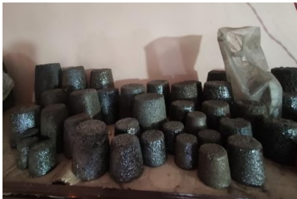
Fig. 3 Various sizes of graphite crucibles are prepared for use in the melting furnace, used to contain and heat metal during the smelting process. Location: workshop of Mr Arjun Kodak, Bageshwar, Uttarakhand, 2023. Photo: Sah and Singh Bhakuni under the ICHR Research Project.
