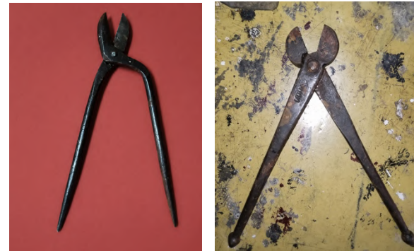
Fig. 10 (left) Kaati, a metal cutting tool used by goldsmiths to trim and cut thin sheets or wires of gold and silver.
