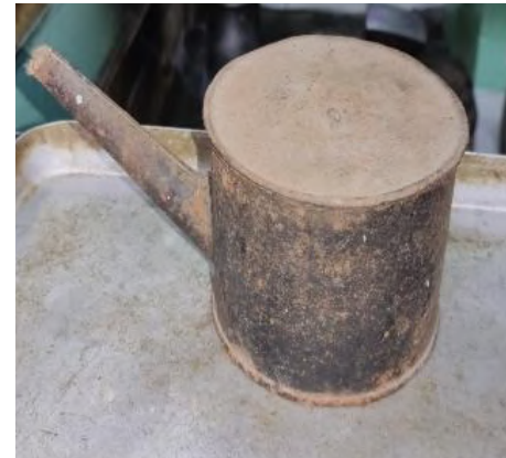
Fig.7 Traditional oil lamp (kuppa) used by goldsmiths to generate flame for melting and heating metals with the help of a banknal.) A goldsmith using a banknal to direct airflow and intensify the flame during the heating and soldering of gold components in the jewellery making process.
