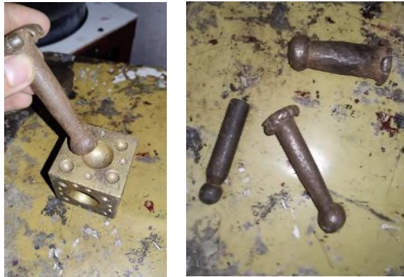
Fig. 22, 23 Wooden and bronze kansala used with iron thukanna of various sizes to shape thin sheets of gold and silver into semi-rounded and domed jewellery components through controlled hammering. Location: workshop of Mr Rajendra Verma, Nainital, Uttarakhand, 2024. Photo: Sah and Singh Bhakuni, 2024, under the ICHR Research Project.
