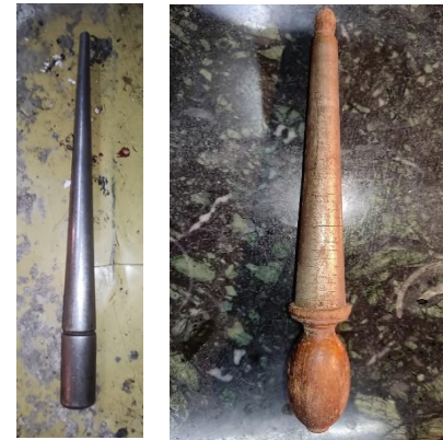
Fig. 24, 25 Ring rod used by jewellers to shape and adjust rings to the required finger size. The tapered rod with size markings helps artisans accurately form and measure rings during the final stages of ring-making. Location: workshop of Mr Rajendra Verma, Nainital, Uttarakhand, 2024. Photo: Sah and Singh Bhakuni, 2024, under the ICHR Research Project.
