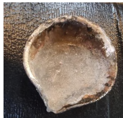
Fig. 4 Clay crucible (ghadiya) used for melting gold, silver, and copper during the jewellery-making process. Location: workshop of Mr Arjun Kodak, Bageshwar, Uttarakhand, 2023. Photo: Sah and Singh Bhakuni under the ICHR Research Project.
