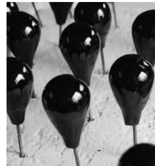
Fig. 22 (left) Surface finishing of porous ceramic elements after demoulding. Photo: Inna Cheskidova.
