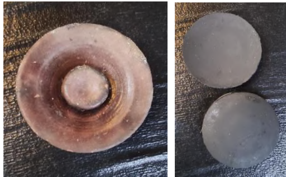
Figs. 8 and 9 Upper and lower components of the clay dabkani, featuring a raised central knob used to apply pressure while flattening gold or silver into thin sheets.
