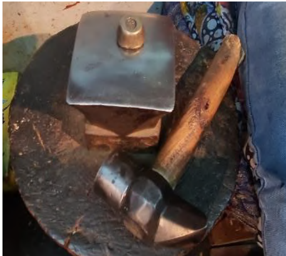
Fig. 18 Traditional hammer and airan used in jewellery-making. The hammer is used to shape and flatten gold or silver, while the iron airan, fixed into a wooden base, provides a stable surface for controlled hammering. Location: workshop of Mr Sudhir Verma, Nainital, Uttarakhand, 2024. Photo: Sah and Singh Bhakuni, 2024, under the ICHR Research Project.
