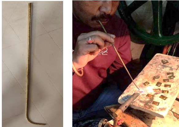
Fig. 5 (left) Banknal, a brass pipe-shaped tool used by goldsmiths to control and direct the flame during the heating and soldering of metals.
