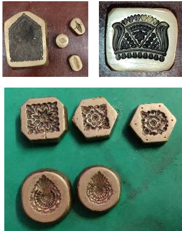
Fig. 19, 20 (top) Traditional metal moulds used in jewellery-making to imprint decorative motifs on gold and silver ornaments. The moulds contain engraved patterns that are transferred onto thin metal sheets through controlled hammering. Location: workshop of Mr Rajendra Verma, Shop no. 211, New Market, Tallital, Nainital, Uttarakhand, 2024. Photo: Sah and Singh Bhakuni, 2024, under the ICHR Research Project.
