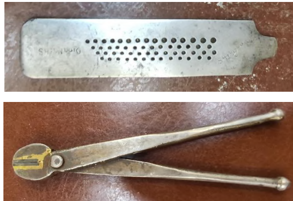
Fig. 14 (top) Jantar , a perforated metal plate used by goldsmiths to draw gold or silver into fine wires of varying thicknesses during the jewellery-making process. Location: workshop of Mr Ram Bharose Lal Verma and Mr Rajesh Kumar Verma, Bada Bazar, Nainital, Uttarakhand, 2024. Photo: Sah and Singh Bhakuni, 2024, under the ICHR Research Project.
