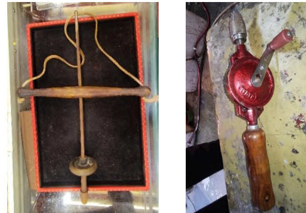
Fig. 16 (left) Traditional baram (hand-operated drill) used in jewellery making for creating fine holes in gold and silver ornaments. Location: workshop of Mr Ram Bharose Lal Verma and Mr Rajesh Kumar Verma, Bada Bazar, Nainital, Uttarakhand, 2024. Photo: Sah and Singh Bhakuni, 2024, under the ICHR Research Project.
