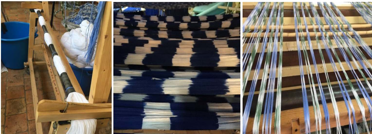
Figure 8. Teixits Viçens, 2018, from left to right: sequence of dyeing cotton thread by resist, drying dyed threads and transfer to the loom for weaving Mallorquí Ikat fabric or cloth of tongues. Photo: S. O'Hana with kind permission from Teixits Viçens
