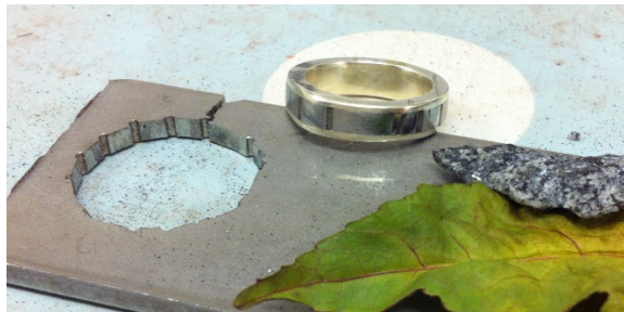
Fig 5: Ring in progress. The steel was inlaid, and the leaves and stone were used to texture the silver. Photo: Rebecca Steiner 2016
