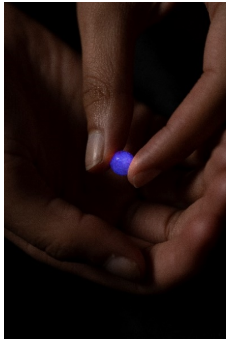
Figure 6 Faceted composite stone (YAG + BRB + YAG) phosphorescing after excitement with UV light source. Photography by Simon Regan for the Centre for Print Research. Image used with kind permission of the Centre for Print Research.
