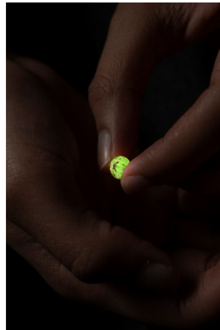
Figure 7 Faceted doublet (YAG + BRG) phosphorescing after excitement with UV light source. Photography by Simon Regan for the Centre for Print Research. Image used with kind permission of the Centre for Print Research.
