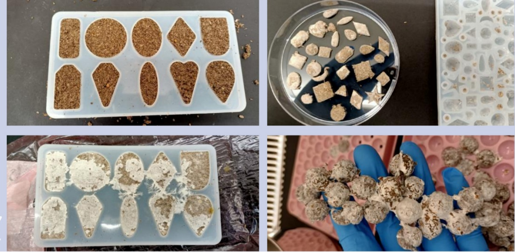
Figure 7 Mycelium growing in Pre-made moulds. Images courtesy of author.
