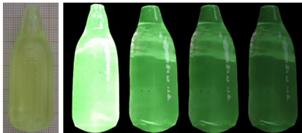
Figure 5 BRG ( \text{Eu}^{2+}, \text{Dy}^{3+}:\text{SrAl}_2\text{O}_4 ) boule. Height = 50 mm. Left, without excitation in natural light. Four boules on the right document the light emission continuously decreasing from excitation to ten hours later. Photography by D. Rytz. Image used with kind permission of D. Rytz.
