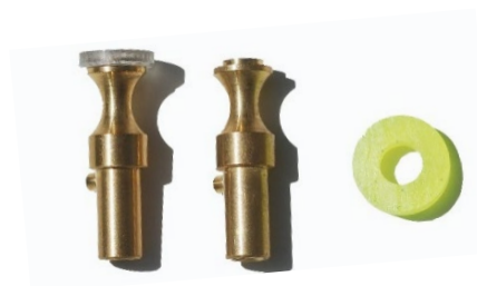
Figure 10 Adapted faceting tools to enable faceting edges of pre-cored BRG material. Image courtesy of author.
