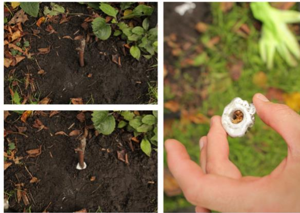
Figures 22-24 anticlockwise starting top left. Figure 22: A stick is implanted into the ground. Figure 23: Molten pewter is poured. Figure 24: The ring's outer and inner textures are formed by that of the ground and the stick respectively. Copyright: Xan Xacobo Goetzee-Barral, 2023.
