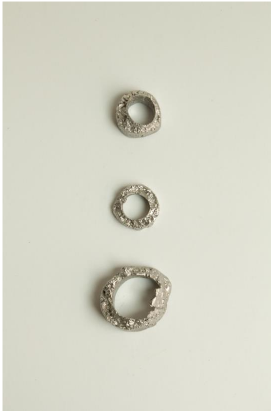
Figure 19: Pewter rings cast by implanting a stick into ground in my back garden to create the mould. Copyright: Xan Xacobo Goetzee-Barral, 2023.
