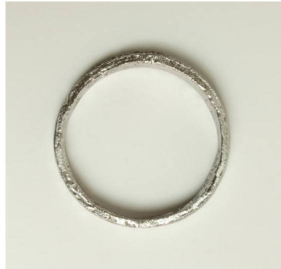
Figure 18: A pewter bangle made by melting three rings (Figure 17) and casting these into hand formed clay. Copyright: Xan Xacobo Goetzee-Barral, 2023.
